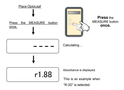
Note: (1) If the selected type of the leaf selection slide switch does not match the actual type of the OptoLeaf to be measured, correct measurement cannot be obtained.
