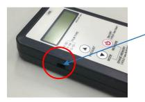
\* If the selected type of the leaf selection slide switch does not match the actual type of OptoLeaf to be measured, correct measurement cannot be obtained.
