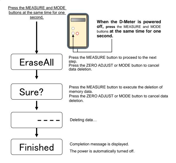
To confirm the deletion, turn on D-Meter and move to the MEMORY mode. If the following (meaning that there is no measurement data) is displayed, it means the data is deleted.
