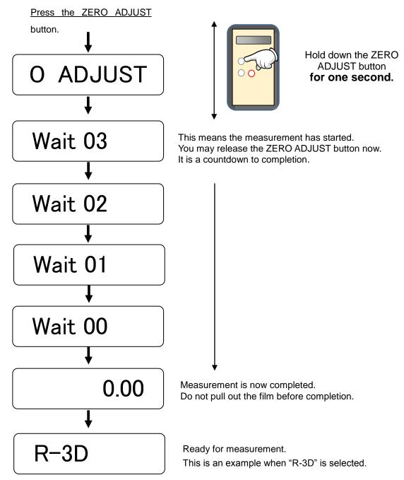
Note: (1) If the ZERO ADJUST switch is released before "Wait 03" is displayed, zero adjustment is canceled. In such a case, the reference used the last time is active.
